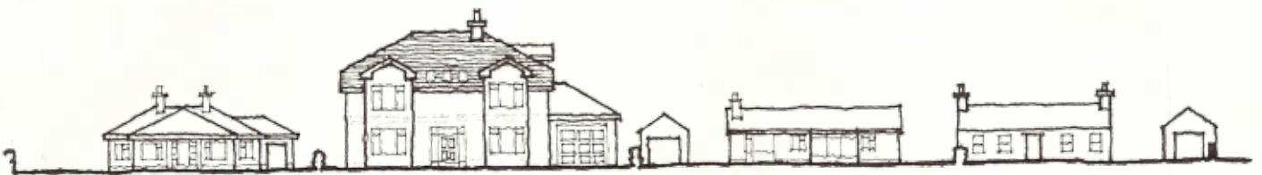
POORLY SCALED ONE HOUSE INFILL TO RIBBON. THIS HOUSE FAILS TO RESPECT THE HEIGHT, SCALE, MASSING + FORM OF ITS NEIGHBOURS.
