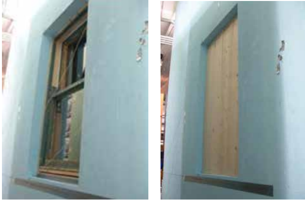
Original Window undergoing test within guarded hot box (University of Ulster)
