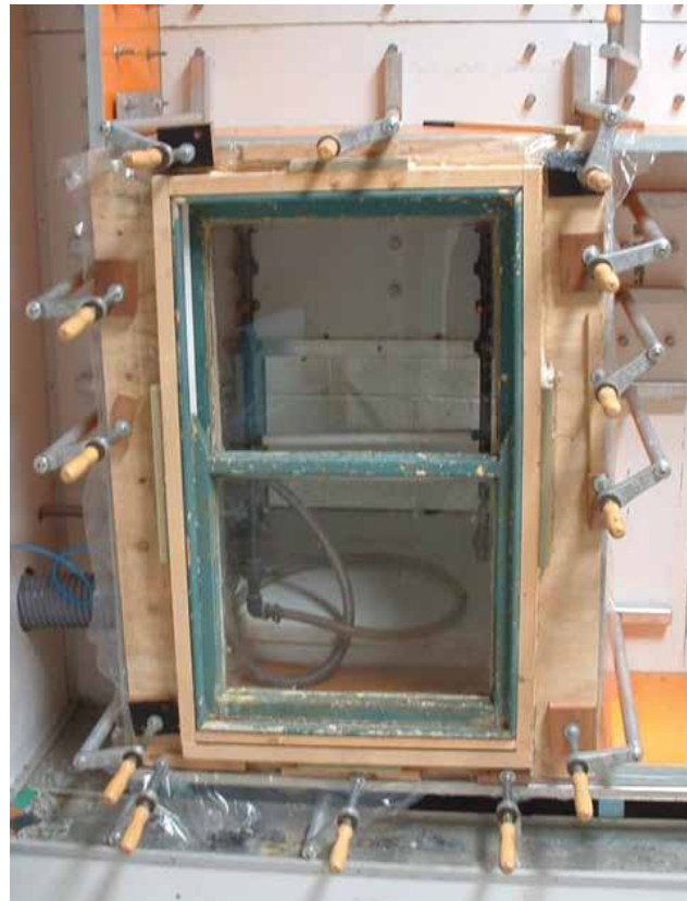
Testing upgraded window in air infiltration test rig Note: position of patent parting bead (University of Ulster)
